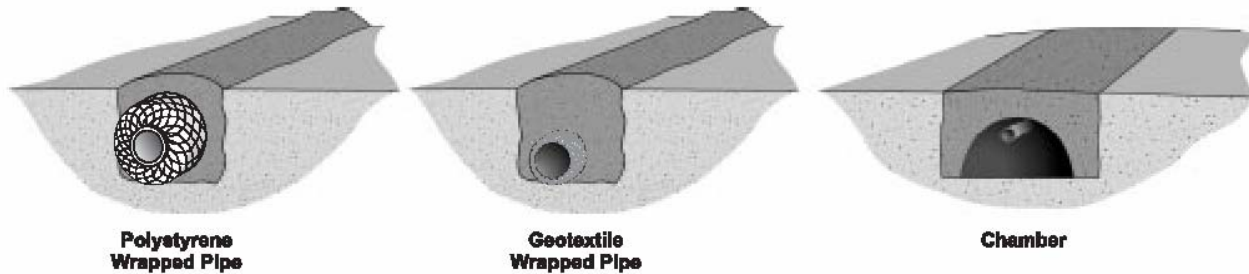
Figure 5: Alternatives to gravel-filled trenches
